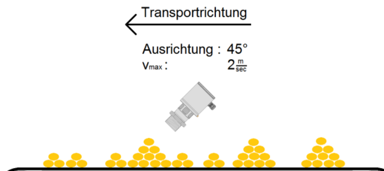
Fig. 11 Mounting on conveyor belt
